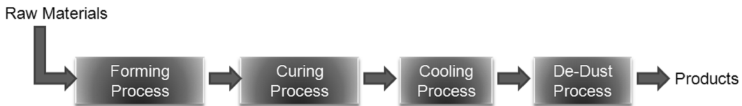
Fig. 1. Glass fiber manufacture process.
