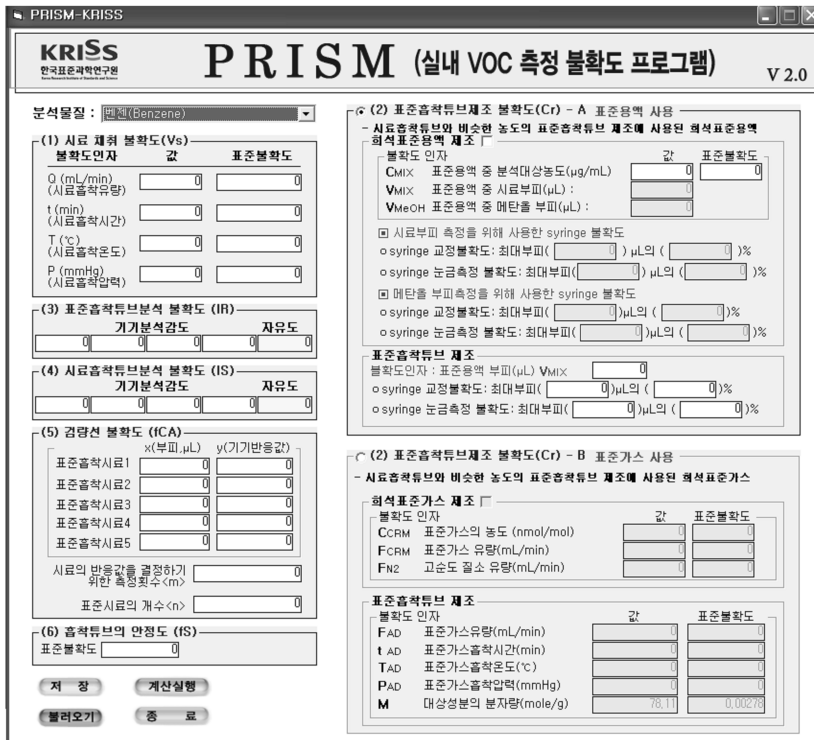
Fig. 1. Uncertainty calculation program(PRISM) for Indoor VOC measurement.
