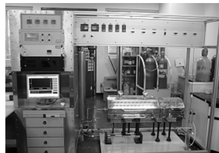
Fig. 2. Catalytic filter test unit.
