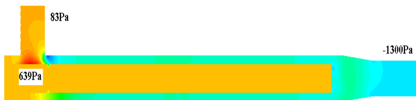
Fig. 5 Pressure in the heating unit
