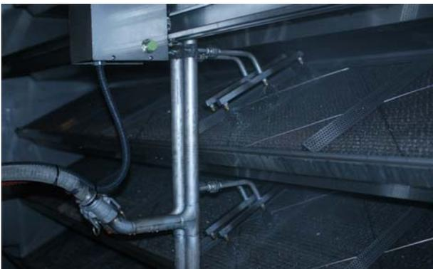
Fig. 5 Filter cleaning by multiple water jet
