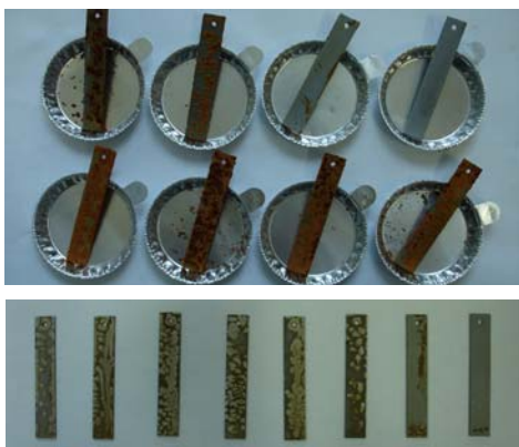
Fig. 4 Photographs of carbon coupons used the batch test.
