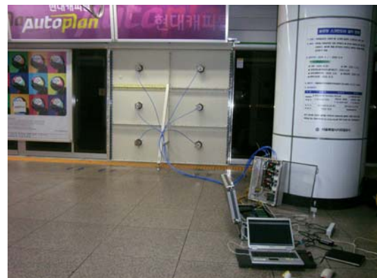
Fig. 4 Measurement of train pressure on PSD
