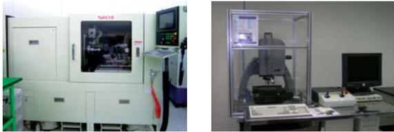
(a) Micro lens processing machine (b) 3D surface measurement system
