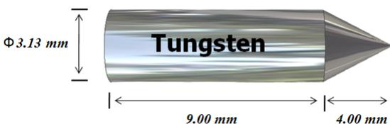
Fig. 1 Electrochemically sharpened tungsten shaft
