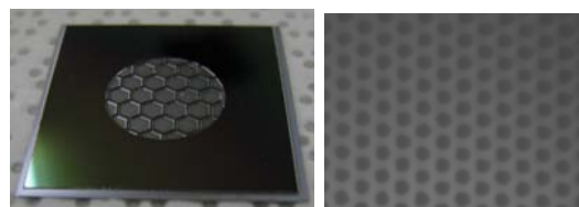
Figure 1 Direct image of porous silicon membrane and SEM image for pore distribution
