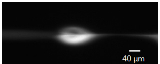
Fig. 4 Janus Particle whose diameter is 50- \mu m. This particle is generated when 10 \mu l/h inner flow rate and 450 \mu l/h outer flow rate are applied.
