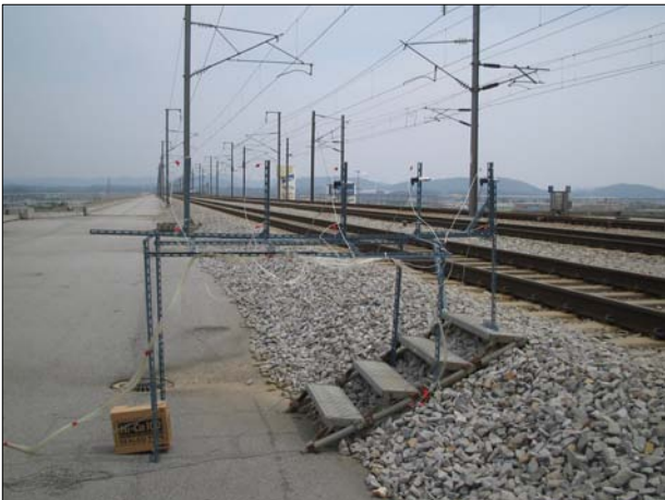
Fig. 6. Field Test of Train Wind Pressure
