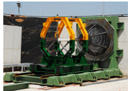
Fig. 5 Thrust Measurement System for High Altitude Simulation Test
