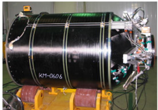
Fig. 7. Thrust axis alignment of KSLV-I KM before ground firing test
