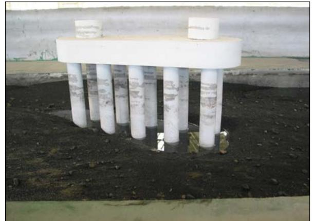
Fig 14. Scouring around a Pier (Physical Result)
