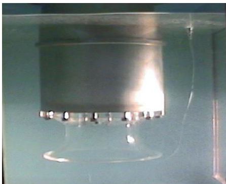
Fig. 3 Observation of the vortex formation in the preliminary test (LLWL, Run-out, AEV)
