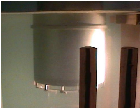
Fig. 8 Observation of thevortex formation in final modification test(LLWL, Run-out, AEV)
