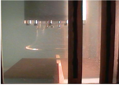
Fig. 6 Observation of the vortex formation in the final modification test(LLWL, Run-out, UGV)
