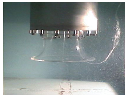
Fig. 2 Observation of the vortex formation in the preliminary test(LLWL, Run-out, UGV)
