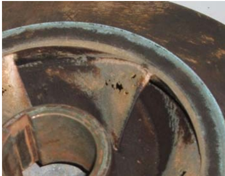
Fig. 4 Impeller damaged by cavitation at excessive capacity
