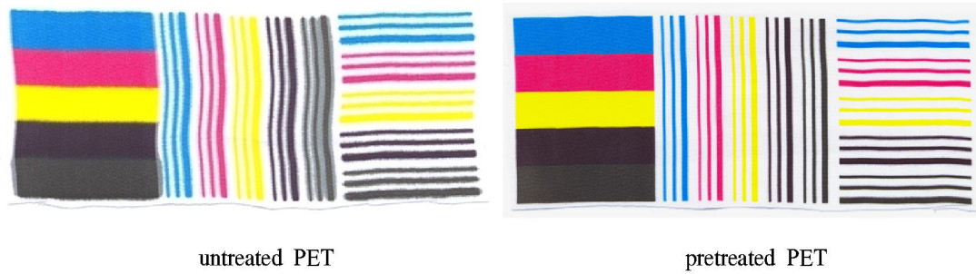
Fig. 1. Effect of digital textile printing on the pretreated and untreated polyester fabrics by media solution.
