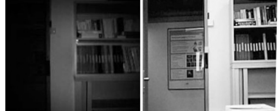
Fig 2. A typical amplitude image delivered by a ToF camera (left), same scene viewed by a webcam (right).
