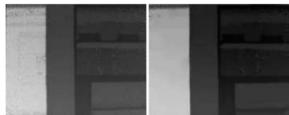
Fig 5. Origin depth image (left). Amplitude-based correction on depth image with amplitude difference map (right).
