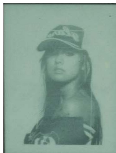
Fig. 3. 4" QVGA e-ink active-matrix displays
