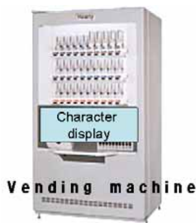
Figure 1 A vending machine image with a CNT-FED character display.
