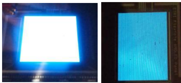
Figure 5. Operating image of top emission AM-OLED on a plastic driven by ZnO TFT.
