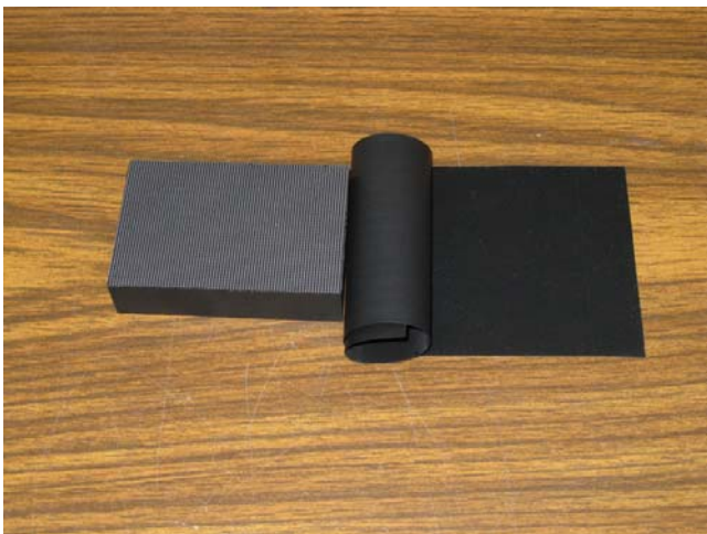
Figure 3. Sample screens on rigid (left) and flexible (right) substrates. The screens appear dark grey under typical indoor lighting conditions since the ambient light is “rejected”.
