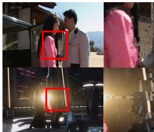
Fig. 1. Example of halo artifacts, left image with original frame and right image magnifying halo artifacts in the interpolated frame
