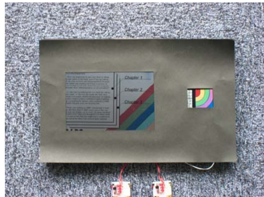
(a) Conventional (b) New reflective LCD Fig. 4 New reflective LCD optimized for large incident light (Incident angle: -45^\circ ).
