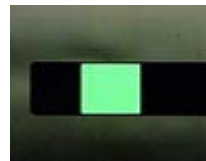
Figure 3. Picture of emitted IBOLED using HNB sputtering process.
