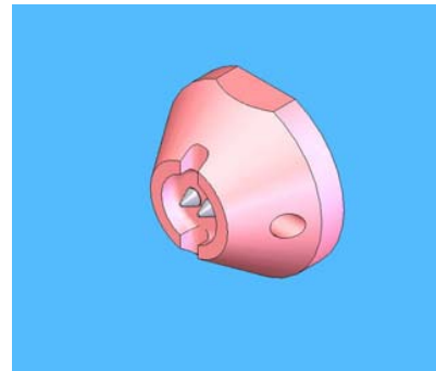
Figure 4: Example of multi (dual) port nozzle that can be employed with a Jet Applicator
