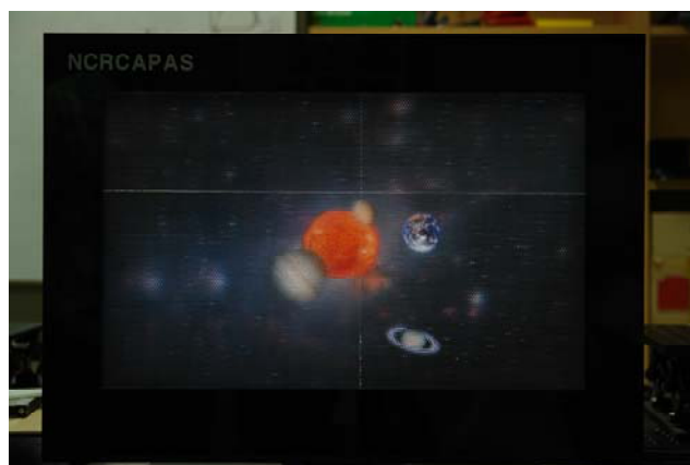
Fig. 2. 22-inch integral imaging system.
