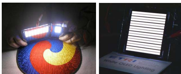
Fig. 7. Photograph of White OLED in this study (100 x 100 mm 2 ).
