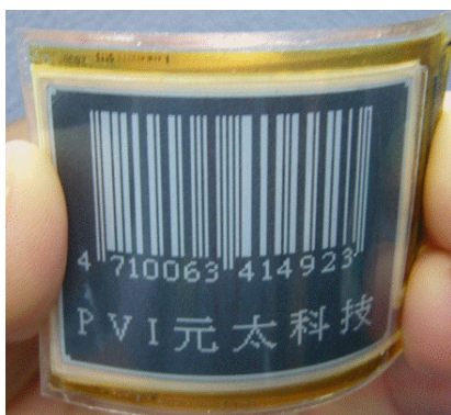
Fig. 4(a) 1.9" Flexi-e display after being addressed and removed from the driving electronics.
