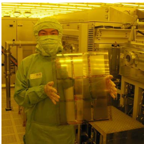
Fig. 1 Photograph of nine Flexi-e TFT arrays on a 370 x 470 mm substrate.
