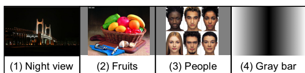
Fig. 3. 4 kinds of test image respectively represent contrast ratio, color shift, luminance and gamma shift image quality in the viewing angle.
