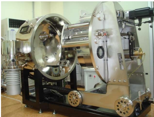
Fig. 1. Picture of a specially designed roll-to-roll(R2R) sputtering system in Kumoh National Institute of Technology
