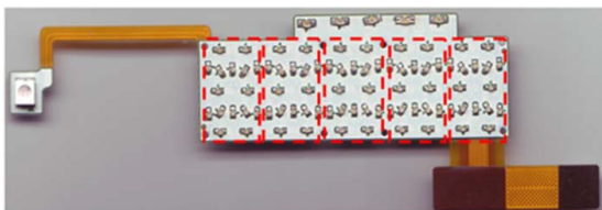
Fig. 8. An actual structure of 5 digits, 16 segments customized display module in mobile application.
