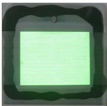
Fig. 1. 2-inch test panel during glow discharge.
