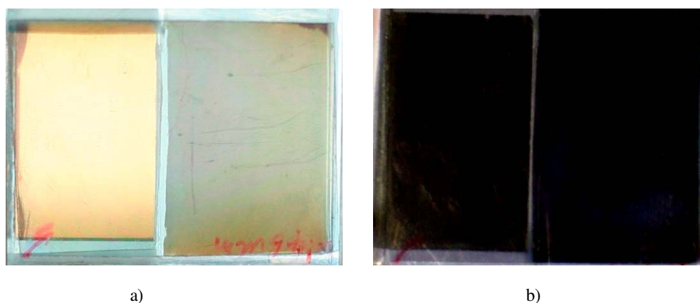
Figure 6 experiment performance with backlighting of a) without voltage and b) with 6V voltage. The reflective part is on the left, the transmissive part is on the right.
