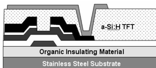
Fig. 1. Device structure of a-Si:H TFT on stainless steel substrate.
