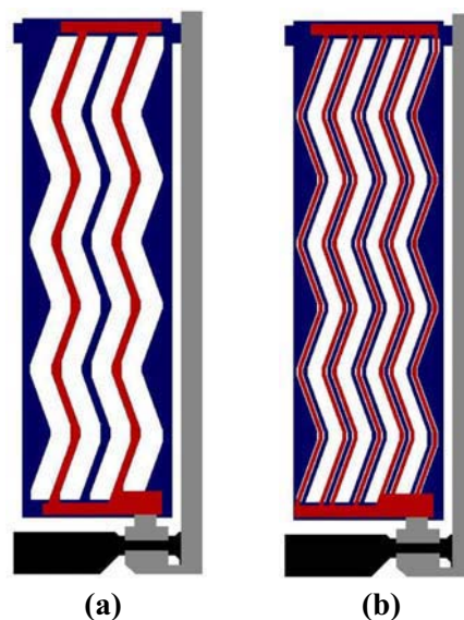
Fig.1. Liquid crystal display cell configuration: (a) conventional S-IPS cell and (b) proposed high transmittance S-IPS cell (Case 2)
