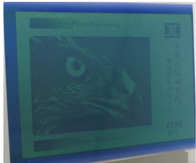
Fig. 7 Laser-addressing result in different initial states.
