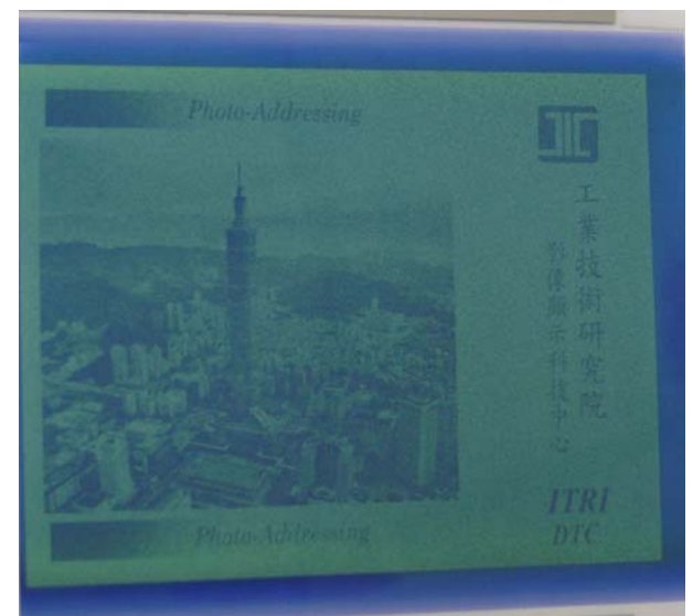
Fig. 9 Laser-addressed images (Panel Size 3.5'' x 4.5'', 300dpi)
