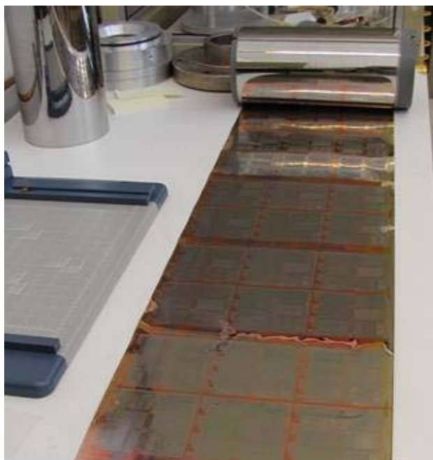
Figure 4. Active matrix backplanes fabricated on continuous 13" wide web. All the steps of film deposition and patterning, along with most of dry and wet etching steps were performed in the R2R environment.
