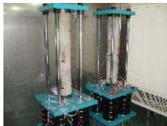
c) strain-gage 부착
