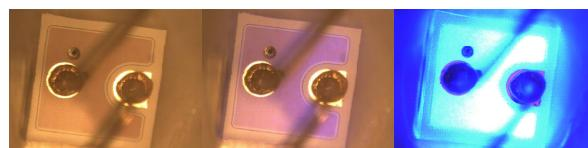
Fig. 8 Failure pattern of LEDs after the MM ESD stress test.
