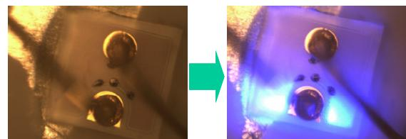
Fig. 6 Failure pattern of LEDs after the HBM ESD stress test.
