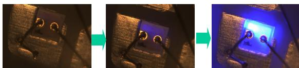
Fig. 4 Failure pattern of LEDs after the reverse over current test.
