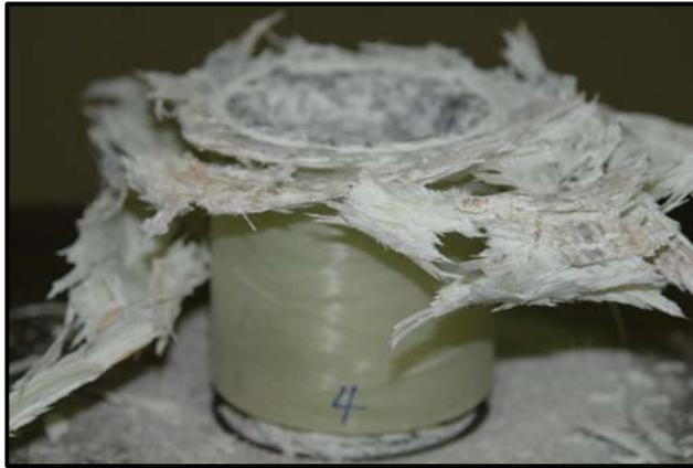
Fig.4 Stable crushing mode for GE3e6
