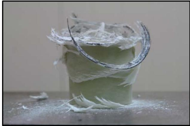
Fig.5 Unstable crushing mode for GE3i4
