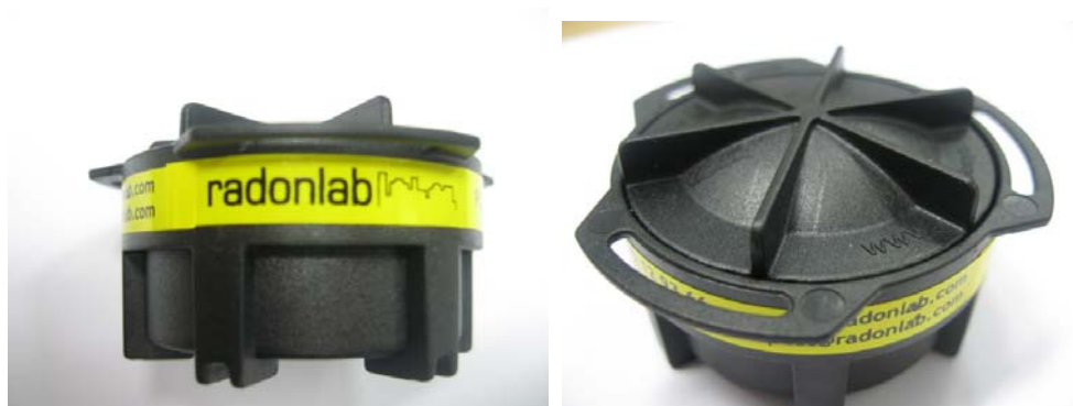
Fig. 7. Radon sampler used in Hong Kong subway
