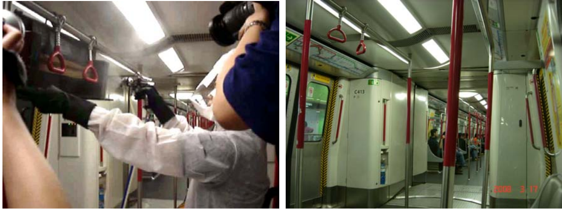
Fig. 5. Photo-catalytic coating by spray and treated knobs (colored by red)
