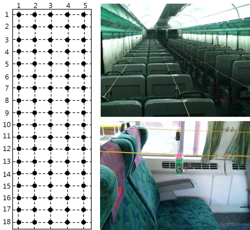
Fig. 2. Sensor node array and pictures of sensor installation
