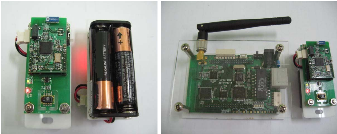
Fig. 1. Sensor node and gateway for data collection
