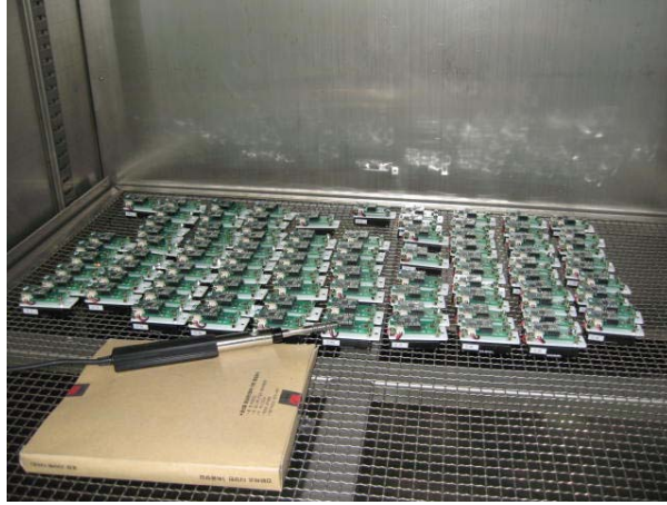
Fig. 3. Temperature and humidity controlled chamber for sensor calibration experiment
