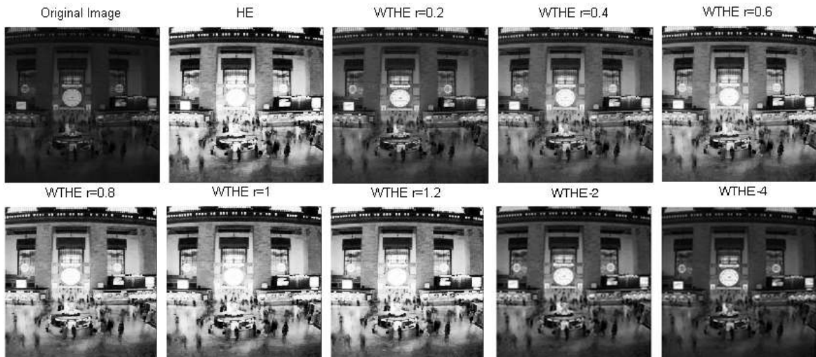
(그림 2) Original/HE/WTHE(r=0.2)/WTHE(r=0.4)/WTHE(r=0.6)/WTHE(r=0.8)/WTHE(r=1)/WTHE(r=1.2) /2WTHE(r1=0.654, r2=0.346)/4WTHE(r1=0.317, r2=0.337, r3=0.243, r4=0.103)
