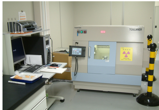
Fig. 1 High resolution micro X-ray computed tomography (CT) system (TOSCNAR 30900µhd, Toshiba co.)
