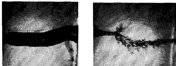
(a)Before PPD application (b) After PPD application 〈Fig. 1〉 Breakdown images by treeing
