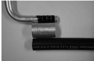
Fig.2 Component of the air-conditioner hose module
