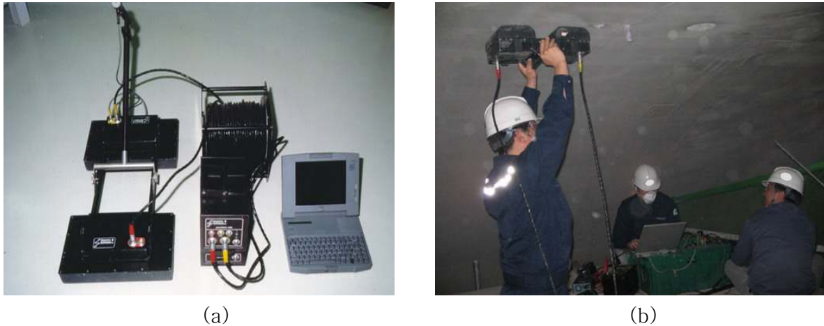
Fig. 1. (a) GPR system(PulseEKKO 1000A™), (b) Data acquisition
