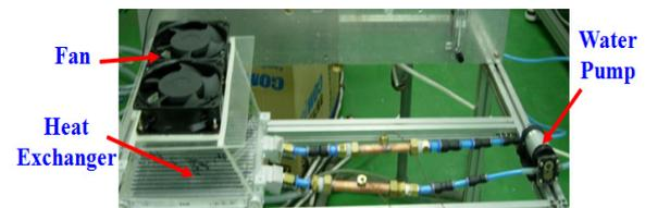
Fig. 7 Water cooling heat exchanger test.
